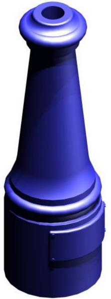
The base has been prototyped with the hole in the centre smaller than required. Using a 1.5mm drill, slowly drill out the hole the full length of the base.
