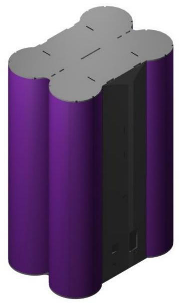
Test fit the top and bottom plates before fitting and clean up any slots and tabs that are tight.
