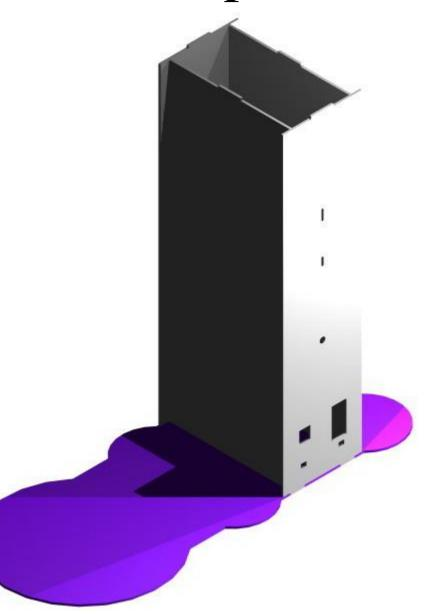
Test fit the top plate before fitting and clean up any slots and tabs that are tight.
